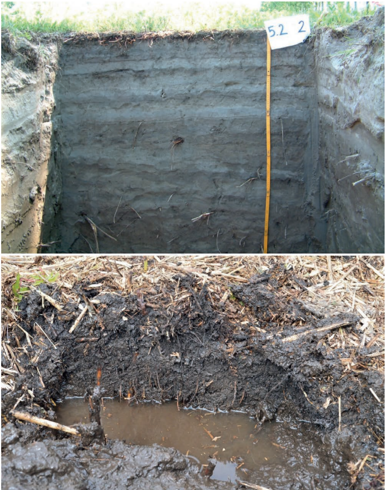
Fig. 8. Upper panel: polyphasic coarse alluvial soil on the Ticino river delta (water table depth of several meters). Lower panel: hydromorphic gley and eutrophic peat soil at the Sabbie d'oro marsh (Brescia: water table depth of 20 cm). Photos credits: L. Giollo (upper panel), N. Patocchi (lower panel).
