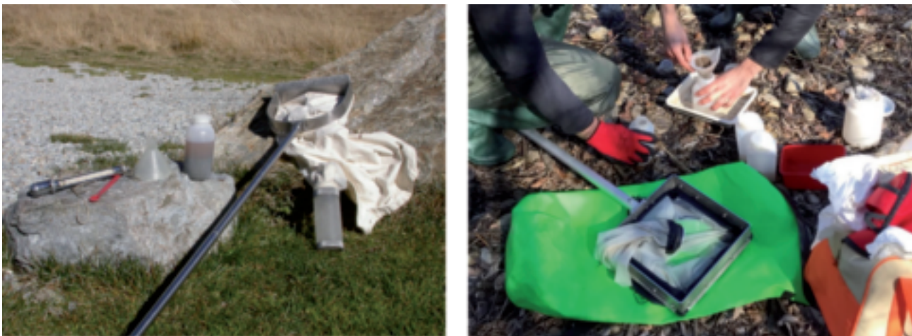
Fig. 3. Handled net, field thermometer, bottle and funnel useful for collecting and treating macro-fauna samples in the field (left). Surber net for collecting meio-fauna samples and filtering procedure (right).
