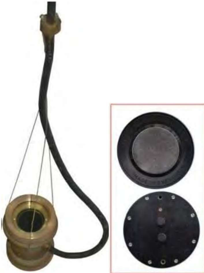
Underwater photometer, Polli type. In the box: two photocells EvansElectroselenium LTD (UK).1952.
