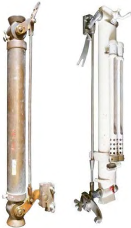
Nansen bottle (left, about 1930) and with support for two reversing thermometers (right, about 1950).
